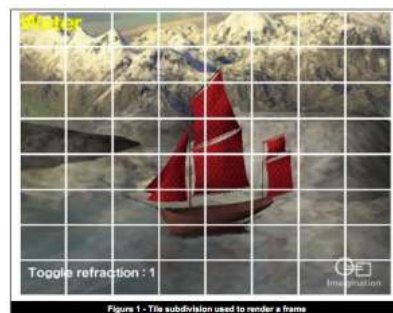
FIGURE 2.17: Screen divided into tiles in tile-based deferred rendering. Source: [KS11].
